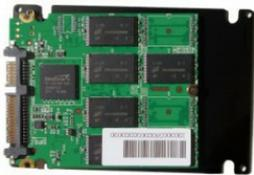
Solid-state drives are currently a bit more expensive than hard disks. However, the use of flash memory instead of disks makes them much lighter and faster than hard disks. SSDs are primarily utilized in portable computers, making them lighter, more durable, and more efficient
