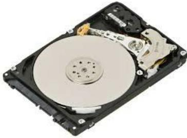
Drives with a capacity less than 1 Terabyte usually have just one platter. Notice the single platter in the image. The read/write arm must be positioned over the appropriate track before accessing or writing data.
