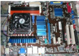
The motherboard is the main circuit board on the computer. The CPU, memory, and storage components, among other things, all connect into the motherboard. Motherboards come in different shapes and sizes, depending upon
